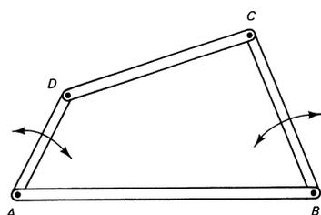
The traditional cycle frame makes use of the triangles strength at the rear, but the main part of the frame BCDE, which supports the front forks, is dependent on the strength of the welds in the joints.
