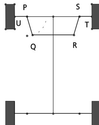
Now it is highly desirable that when taking a bend, the four circles to which the tyres are tangents should all have the same centre - otherwise the front tyres will soon lose their tread. The design problem is to choose  $p$  and  $q$  so that the point  $V$  of intersection of the stub axles produced lies as close to the line  $AW$  as possible for all positions of  $Q$ . Of course there also physical constraints on the maximum sizes of  $p$  and  $q$ .
