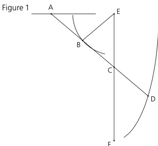
Here the door is represented by  $AD$ . The bar  $EB$  is free to rotate about the top of the door frame  $E$ , and a
